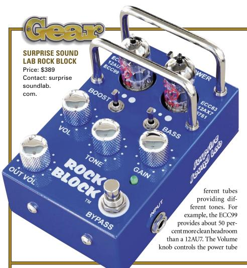
while the Gain controls the preamp tube. When used as a distortion pedal, the Rock Block provides output-tube distortion by using the internal output transformer and an internal speaker load.
