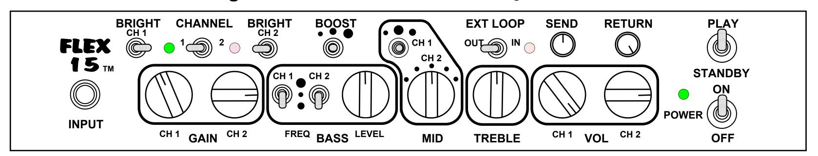
Single Coil CH1: Moderate Overdrive CH2: High Gain
